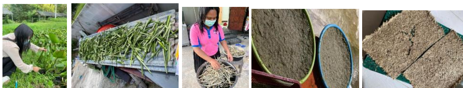
Figure 1 Process to prepare cushioning materials from water hyacinth
