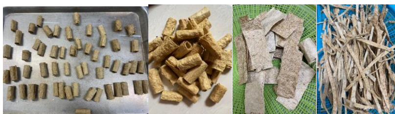
Figure 2 Process to prepare cushioning materials from bagasse
