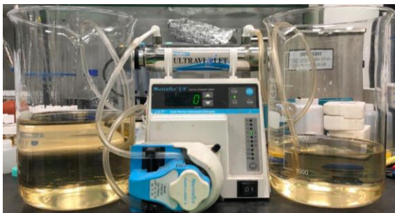
Fig. 2 Experimental setup of UV disinfection.
