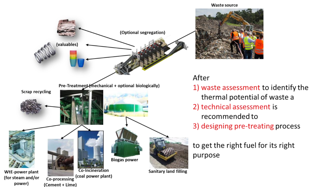
Fig. 1: The strategy and goal(s) must be defined in advance to determine the solution as well as the financial requirements for a meaningful and sustainable operation.
